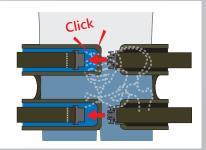
Hold the left and right straps and pull them in opposite direction. < It is recommended that the upper and lower straps be pulled simultaneosly in opposite direction by two people.>
